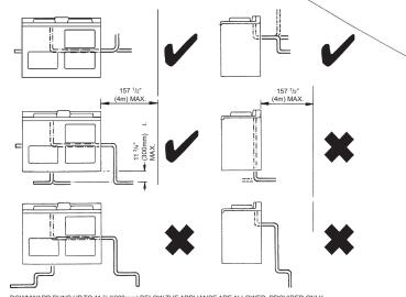
DOWNWARD RUNS UP TO 11  $^3/a^{\circ}(300 mm)$  BELOW THE APPLIANCE ARE ALLOWED, PROVIDED ONLY ONE BEND IS USED.
